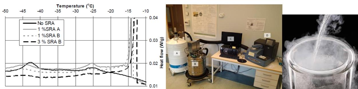
Figure 1. LTC scans for cement paste with different dosage of SRA<sup>3</sup>. LTC equipment.
